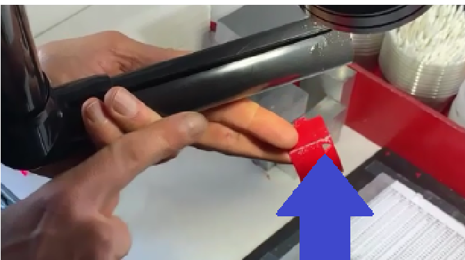
2. Point small triangle towards end of pipe.
