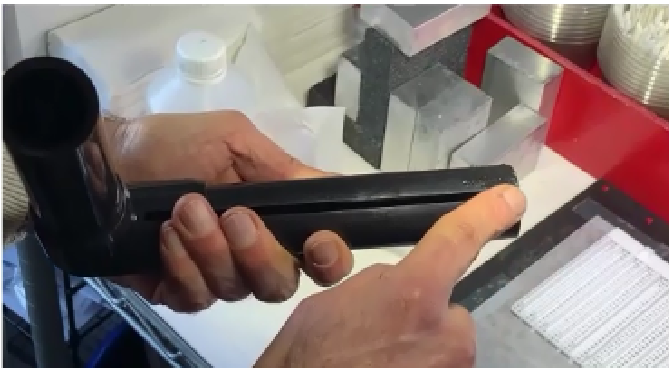
1. Clean with alcohol and apply thin coat of silicone.
