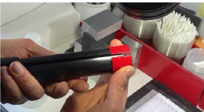
3. Put on pipe and line up slots.
