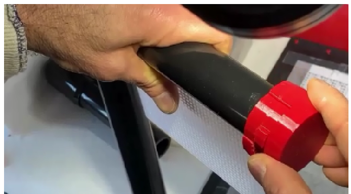
6. After drying overnight, push on cap and turn right.
